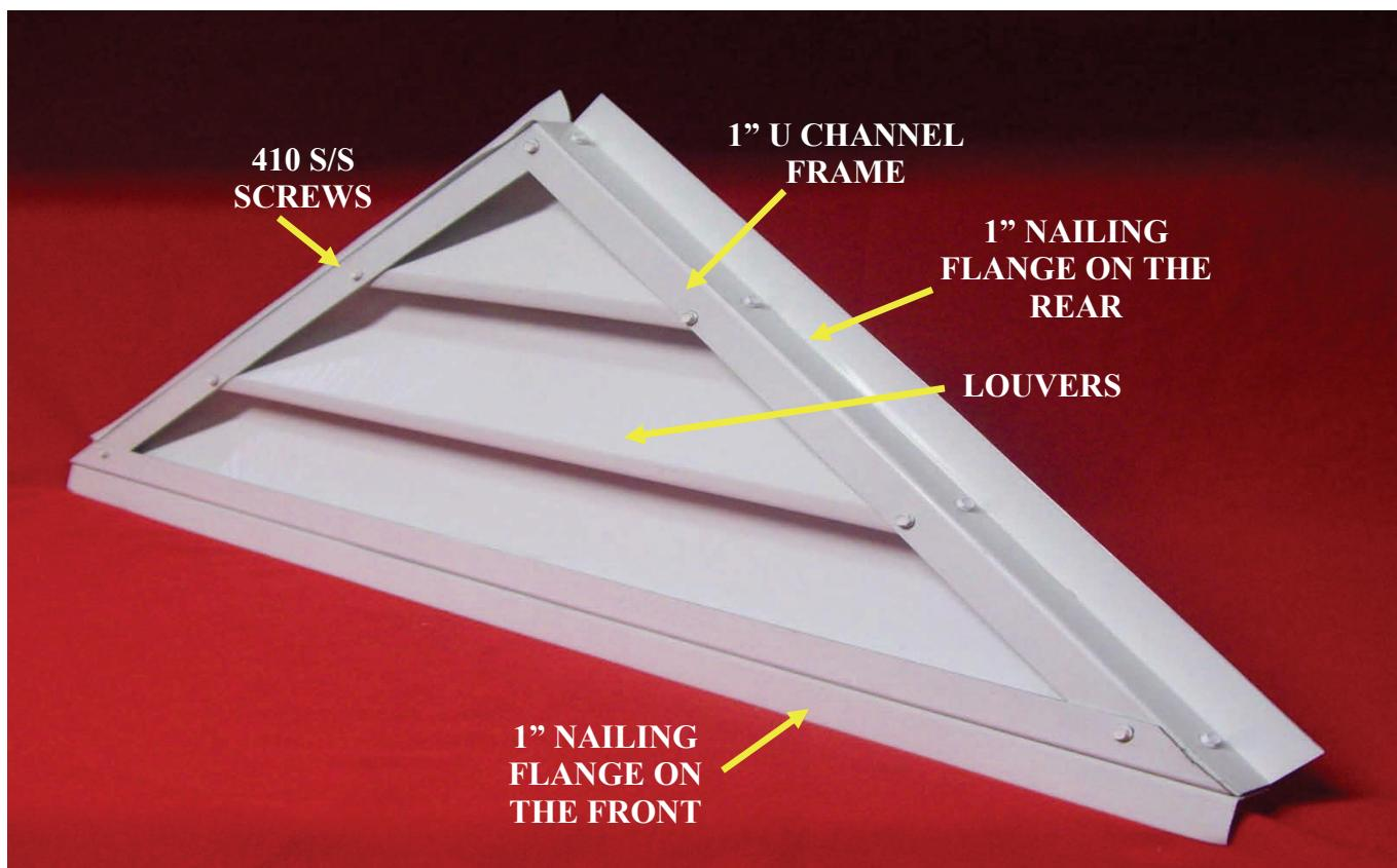
Custom made to fit your opening. Triangle, Square, Rectangle or custom to your pattern. (no 1/2 rounds or circle tops) The nail fin can go on the front side or rear. The nail fin can be field reversed or left off completely. The louvers are .024 thickness and the U-Channel frame is an .040 thickness with a baked on enamel finish. Aluminum screen mesh is standard on the back of all vents. They come in two colors white or antique white.
